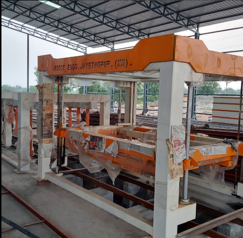
WIRE CUTTING MACHINE
